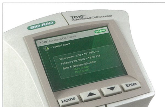
Fig. 3. Current count screen showing a total cell count (without trypan blue dye).
